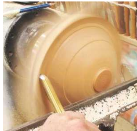
▲ Pic.12 I find it's best to work each shape by doing a bit on one side, followed by a bit on the other. My right hand has to go towards the floor during the cut; this raises the cutting tip and keeps the bevel of the tool in contact with the wood
